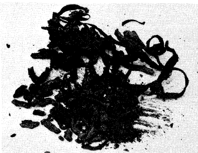
Fig. 3 Charred remains of parachute after ignition during drop test at Sandia Labs., Tonopah Test Range, Nevada.
